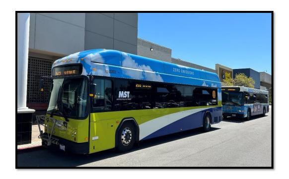
Electric vehicles have several challenges in Monterey County. The distances of MST's rural routes are beyond the capacity of current batteries, which last for about 135 miles or 5 hours, significantly less than a bio fueled heavy duty bus. Even city routes require the electric vehicles to be rotated before a regular eight-hour shift. More charging stations and larger-capacity batteries are likely in the future.
